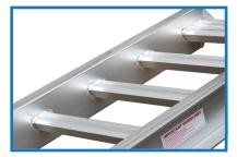
Rungs: High tensile aluminium extrusions. 530mm wide, set down 60mm into the side beams. They have two ribs on the top surface, designed for superior traction.
