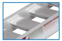
Rungs: High tensile aluminium extrusions. 300mm wide, set down 30mm into the side beams. They are serrated on the top surface, designed for superior traction.
