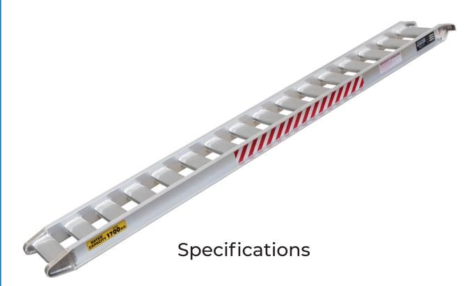
Length: 3000mm. Suitable for deck heights between 1000mm - 1080mm Capacity: 1700kg (axle load across the pair) Weight: 22kg each
