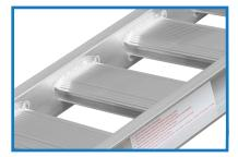
Rungs: High tensile aluminium extrusions. 300mm wide, set down 20mm into the side beams. They are serrated on the top surface, designed for superior traction.
