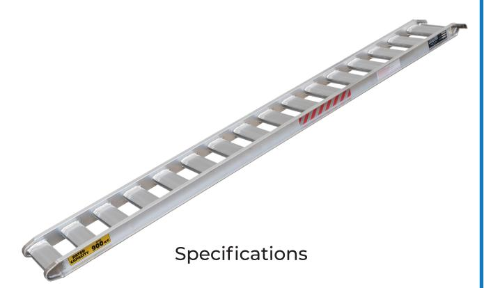
Length: 3000mm. Suitable for deck heights between 1000mm - 1080mm Capacity: 900kg (axle load across the pair) Weight: 19kg each
