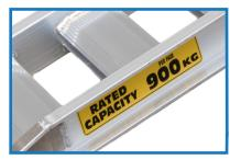
Capacity: These ramps are rated for a 900kg axle load rating across the pair. The rated capacity must exceed the heaviest axle or concentration of load.
