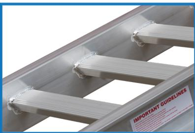
**Rungs:** High tensile aluminium extrusions. 530mm wide, set down 40mm into the side beams. They are serrated on the top surface, designed for superior traction.
