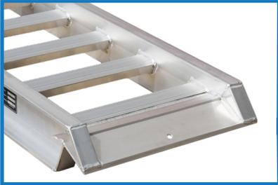
**Headplate:** The 125/330 ramps have a 90mm headplate which sits on the back of your truck deck. The headplate is positioned for a 20° loading gradient.
