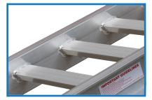
Rungs: High tensile aluminium extrusions. 530mm wide, set down 45mm into the side beams. They are serrated on the top surface, designed for superior traction.
