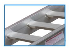
Rungs: High tensile aluminium extrusions. 530mm wide, set down 45mm into the side beams. They are serrated on the top surface, designed for superior traction.
