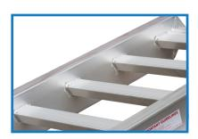
Rungs: High tensile aluminium extrusions. 600mm wide, set down 60mm into the side beams. They are serrated on the top surface, designed for superior traction.
