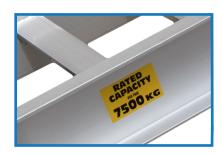
Capacity: These ramps are rated for a 7500kg axle load rating across the pair. The rated capacity must exceed the heaviest axle or concentration of load.
