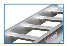
Rungs: High tensile aluminium extrusions. 430mm wide, set down 45mm into the side beams. They have two ribs on the top surface, designed for superior traction.
