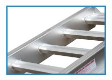
Rungs: High tensile aluminium extrusions. 430mm wide, set down 45mm into the side beams. They have two ribs on the top surface, designed for superior traction.
