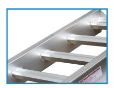
Rungs: High tensile aluminium extrusions. 600mm wide, set down 60mm into the side beams. They have two ribs on the top surface, designed for superior traction.
