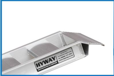
**Headplate:** The L70 150 ramps have a 60mm headplate which sits on the back of your truck deck. The headplate is positioned for a 23° loading gradient.
