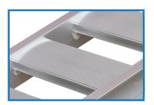
Rungs: High tensile aluminium extrusions. 300mm wide, set down 6mm into the side beams. They are serrated on the top surface, designed for superior traction.
