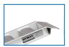
Headplate: The L70 240 ramps have a 90mm headplate which sits on the back of your truck deck. The headplate is positioned for a 20° loading gradient.
